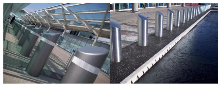
The OZTIME 40 SUPER SHALLOW MOUNT is an ultra shallow foundation static bollard tested at Mira with the N2 7.5 ton vehicle at 64kph. This bollard requires a foundation depth of just 125mm meaning you can easily avoid all ground based services. The unique and simple nature used to connect the bollards means that it can be installed in cambers and gradients.
