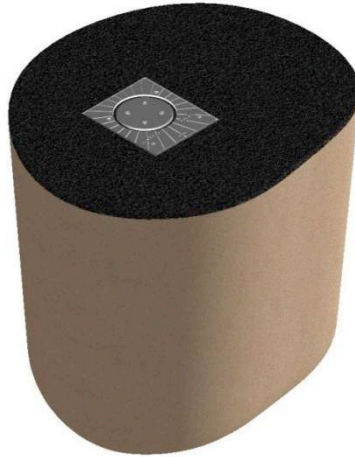
Figure 32: Finished top layer completed with asphalt
