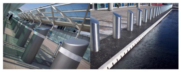
The OZTIME 40 SUPER SHALLOW MOUNT is an ultra shallow foundation static bollard tested at Mira with the N2 7.5 ton vehicle at 64kph. This bollard requires a foundation depth of just 125mm meaning you can easily avoid all ground based services. The unique and simple nature used to connect the bollards means that it can be installed in cambers and gradients.
